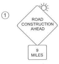
1 IL Route 96/900N W20-I103 (O) 48 W16-3 (O) 3024 Type A Flashing Light
