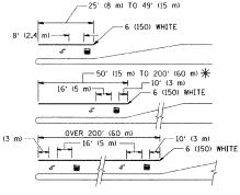
FULL SIZE LETTERS 8' (2.4 m) AND ARROWS SHALL BE USED. AREA = 15.6 SO. FT. (1.5 m<sup>2</sup> ) (11.5 m<sup>2</sup> ) (11.9 m<sup>2</sup>)
