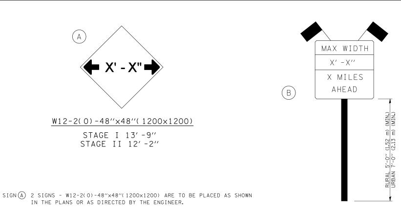
SIGN (B) 2 SIGNS - (SIGN PANEL, TYPE II) AS SHOWN ARE TO BE PLACED AS SHOWN IN THE PLANS OR AS DIRECTED BY THE ENGINEER.
