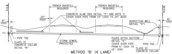
STORM SEWER LESS THAN 2' (600 mm) BELOW DITCH FLOW LINE AND STORM SEWERS CROSSING UNDER PAVEMENTS AND PAVED DITCHES
