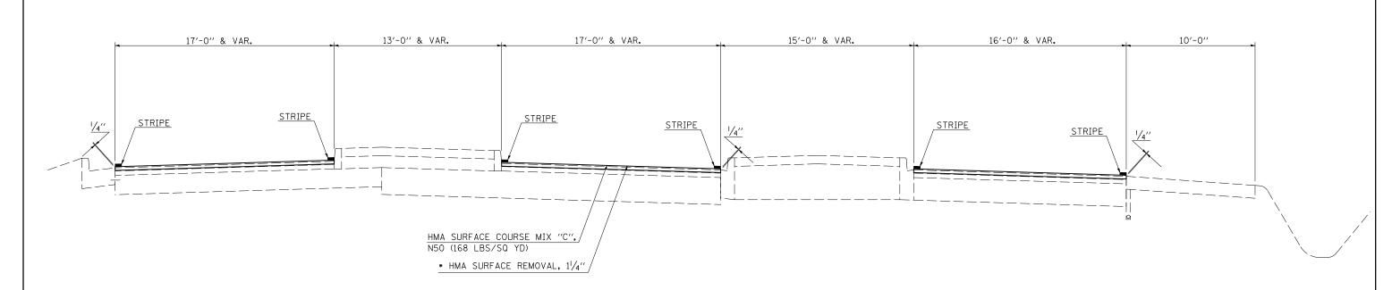
\* REMOVE A MAXIMUM OF 11/4" SURFACE MATERIAL ACROSS THE PAVEMENT IN ORDER TO AVOID DAMAGE TO THE EXISTING CRACK CONTROL TREATMENT.
