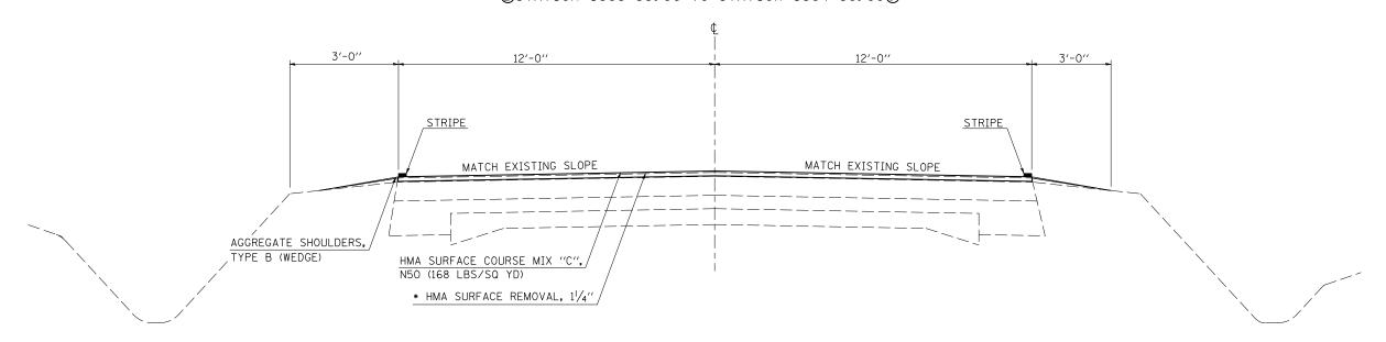
\* REMOVE A MAXIMUM OF 11/4" SURFACE MATERIAL ACROSS THE PAVEMENT IN ORDER TO AVOID DAMAGE TO THE EXISTING CRACK CONTROL TREATMENT.
