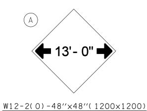
SIGN (A) 2 SIGNS - W12-2(0)-48"×48"(1200×1200) ARE TO BE PLACED AS SHOWN IN THE PLANS OR AS DIRECTED BY THE ENGINEER.
