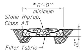
**SECTION B-B THRU RDWY. EMBANKMENT**
