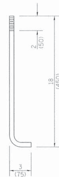
ANCHOR ROD DETAIL
