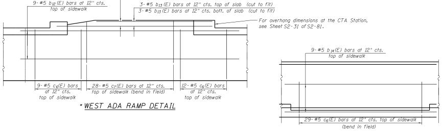
\* See Roadway Plans for ADA Ramp slope and ADA Ramp layout
