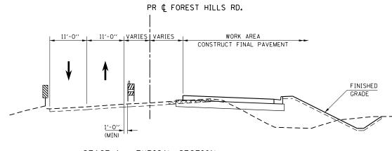
STAGE 1 - TYPICAL SECTION STA 453+22.84 TO STA 455+55.00
