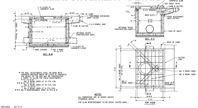
INLET SPECIAL NO. 3, 4, 5, 6 REINFORCEMENT DETAIL 79.4q **INLET SPECIAL NO. 7 & 8 REINFORCEMENT DETAIL**
