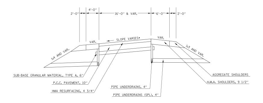
\* SLOPE VARIES IN SUPERELEVATION AREAS WITH A MAXIMUM OF 8.0% DIFFERENCE IN PAVEMENT GRADE AND SHOULDER GRADE.
