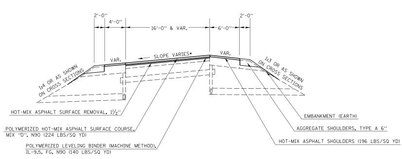
\* SLOPE VARIES IN SUPERELEVATION AREAS WITH A MAXIMUM OF 8.0% DIFFERENCE IN PAVEMENT GRADE AND SHOULDER GRADE.
