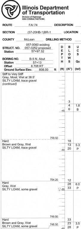
The Unconfined Compressive Strength (UCS) Failure Mode is indicated by (B-Bulge, S-Shear, P-Penetrometer) The SPT (N value) is the sum of the last two blow values in each sampling zone (AASHTO T206)
