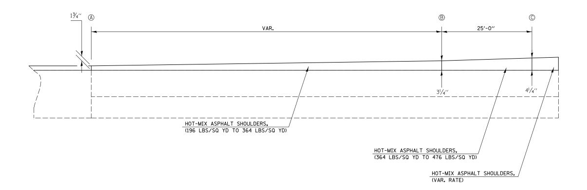
\* HOT-MIX ASPHALT SURFACE REMOVAL, BUTT JOINT WILL BE REQUIRED FOR RAMP N FROM STA. 24+62.00 TO STA. 21+24.00 (VAR. DEPTH)
