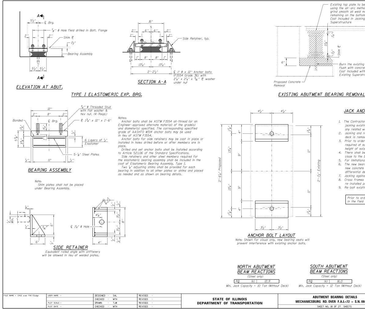
Existing top plate to be removed using the air-arc method and grind smooth all weld material remaining on the bottom flange. Cost included in Jacking Existing Superstructure
