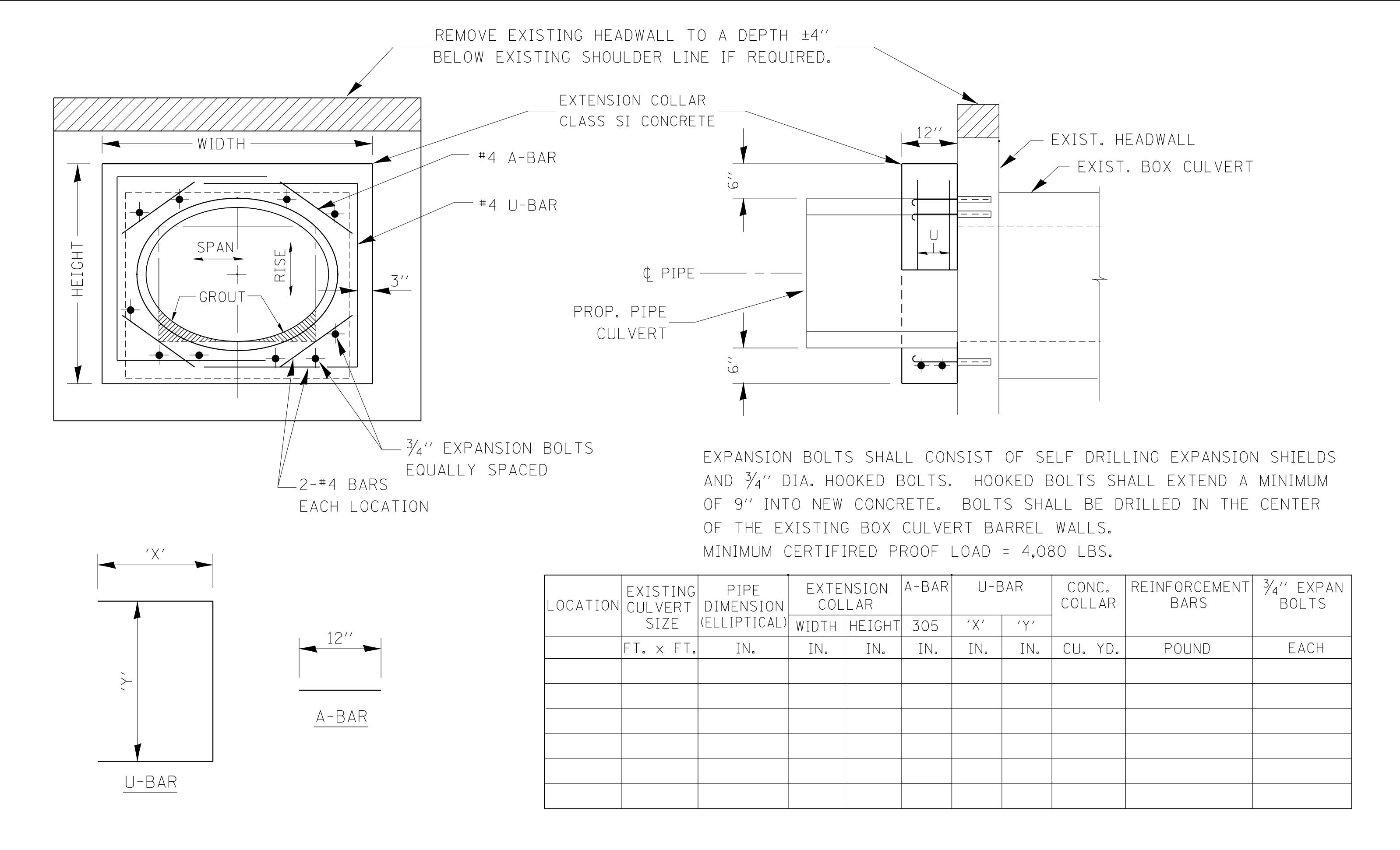
COLLAR DETAIL (ELLIP. CONC. EXTENSION OF BOX CULVERT)
