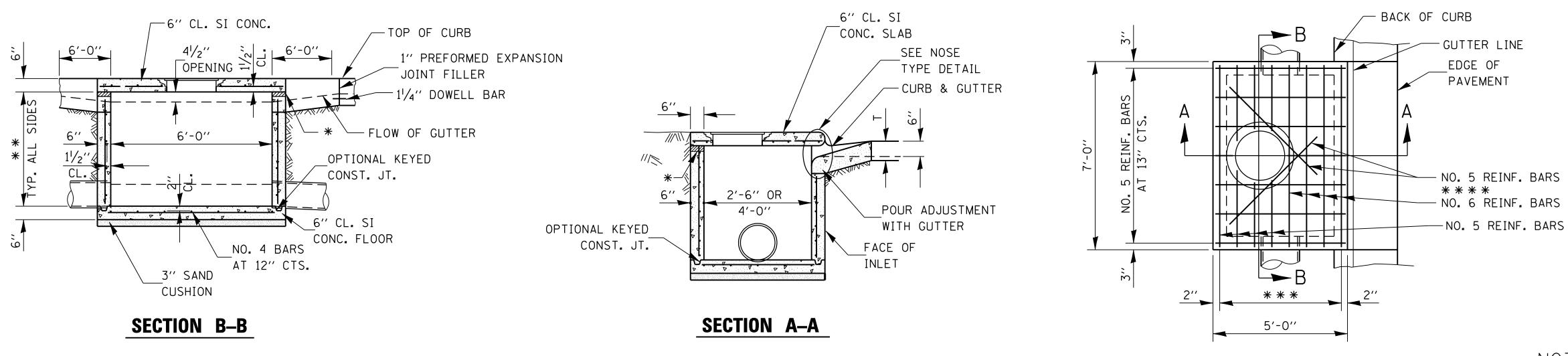
TOP SLAB REINFORCEMENT TO BE EPOXY COATED BARS.
