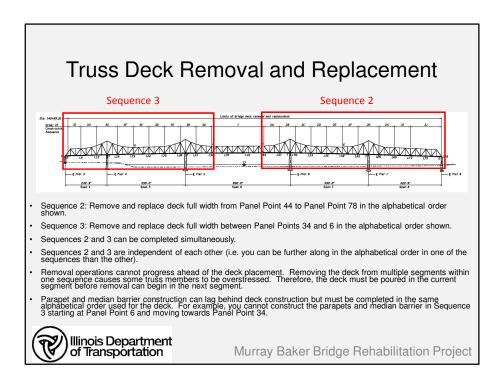
Once the removal and replacement over the suspended span is complete, you would move on to Sequences 2 and 3. Sequence 2 is the removal and replacement from Panel Point 44 to Panel Point 78. Sequence 3 is the removal and replacement from Panel Point 34 and working back towards Panel Point 6.
