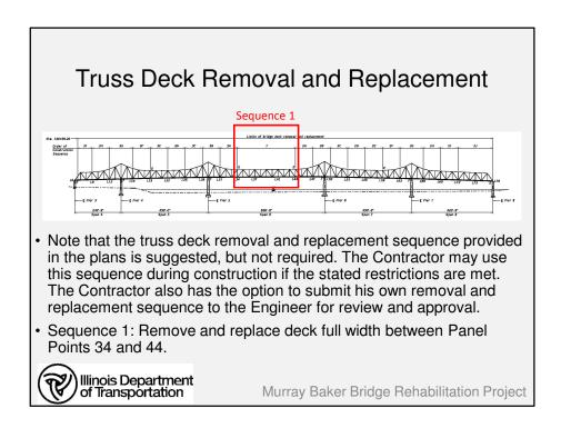
Note that the truss deck removal and replacement sequence provided in the plans is suggested, but not required. The Contractor may use this sequence during construction if the stated load restrictions are met. The Contractor also has the option to submit his own removal and replacement sequence to the Engineer for review and approval.
