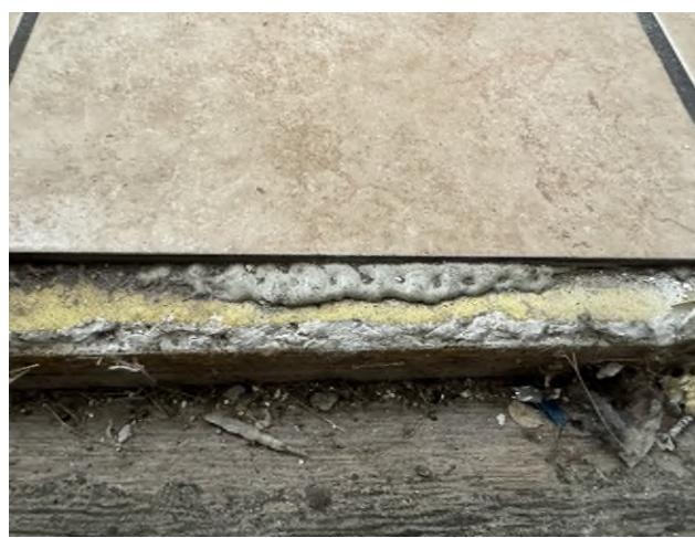
HA-7: Tan with Red Tint 12" x 12" Ceramic Tile; HA-8: Gray Adhesive associated with HA-7 HA-9: Black Grout associated with HA-7
