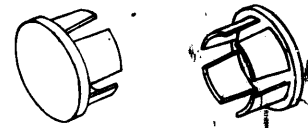
CAST END CAP DRIVE FIT TYPE 12 Required Galvanize to A.S.T.M. A-153. Incidental to item "Metal Handrail".
