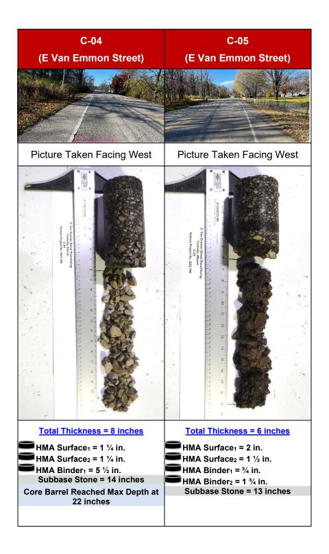
The referenced thicknesses are considered approximate. Commentary provided by Rubino is based on our observation in the laboratory; **Crack** = vertical through cross section; **Weathering** = rounded edges & degradation of asphalt and **Deterioration** = horizontal crack. Pavement and subbase type and thickness may vary between core locations. Any comments on the condition of the material are considered our opinion and should be verified by the design engineer.
