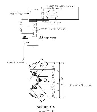
DETAIL OF CONNECTION OF GUARDRAIL TO SQUARE BRIDGE PIER OR FOUNDATION.
