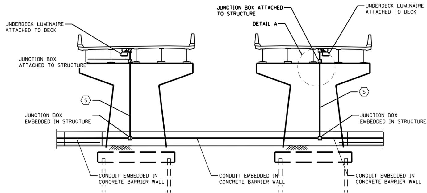
**PIER ELEVATION - SECTION A-A**
