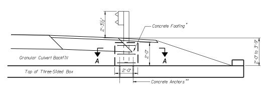
ANCHORED WITH CONCRETE FOOTING AND ATTACHED TO TOP OF BOX
