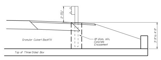
ANCHORED WITH CONCRETE ENCASEMENT
