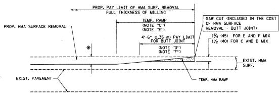
HMA CONSTRUCTED TEMPORARY RAMP (FOR BUTT JOINT AND HMA TAPER SEE DETAIL BELOW)
