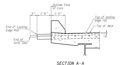
The pay items for Preformed Joint Strip Seal shall be to the end of the steel plate. The 6" of rubber extending past the end of the steel shall be considered incidental and and shall not be measured for payment.
