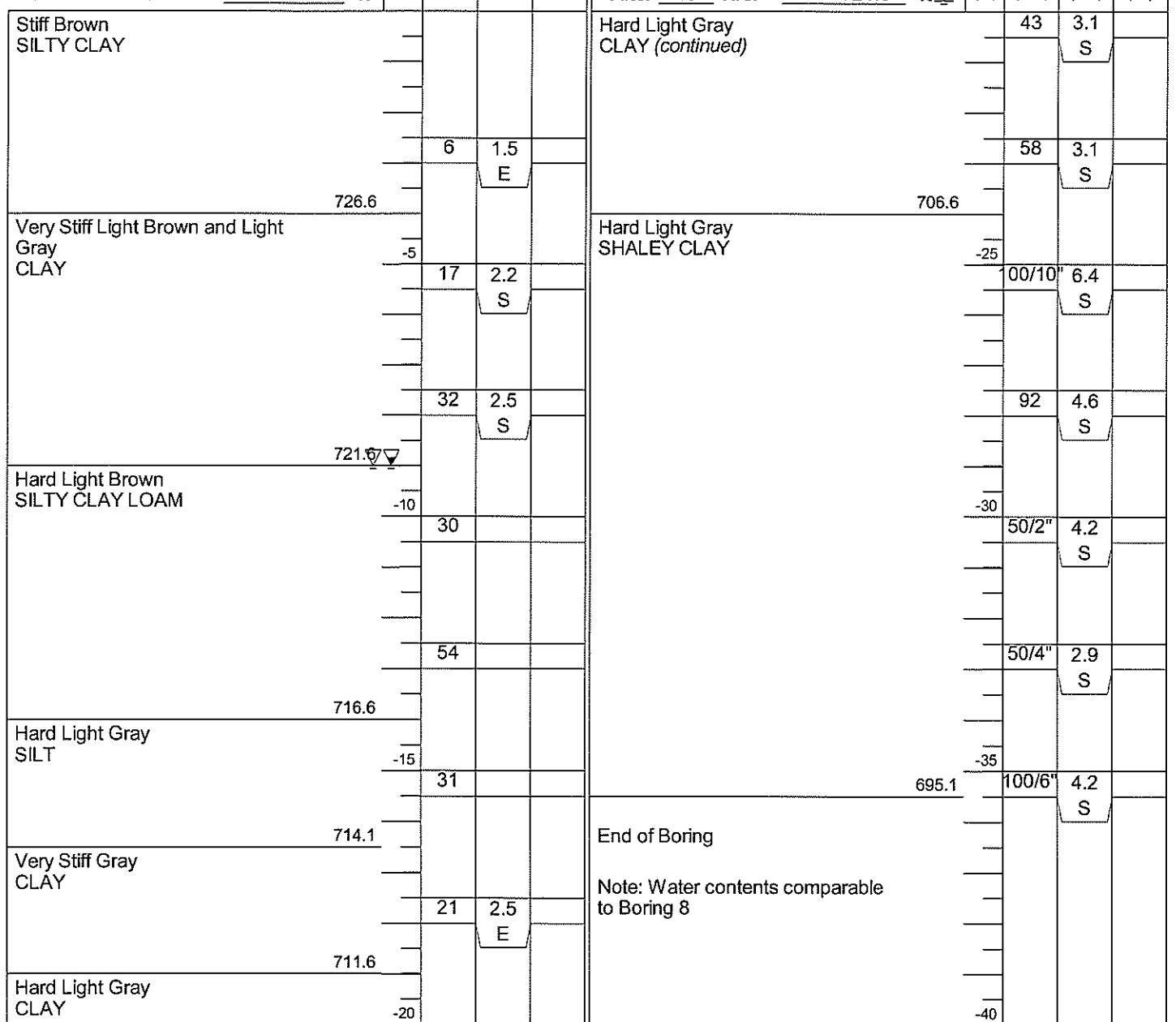
The Unconfined Compressive Strength (UCS) Failure Mode is indicated by (B-Bulge, S-Shear, P-Penetrometer). The SPT (N value) is the sum of the last two blow values in each sampling zone (AASHTO T206).
