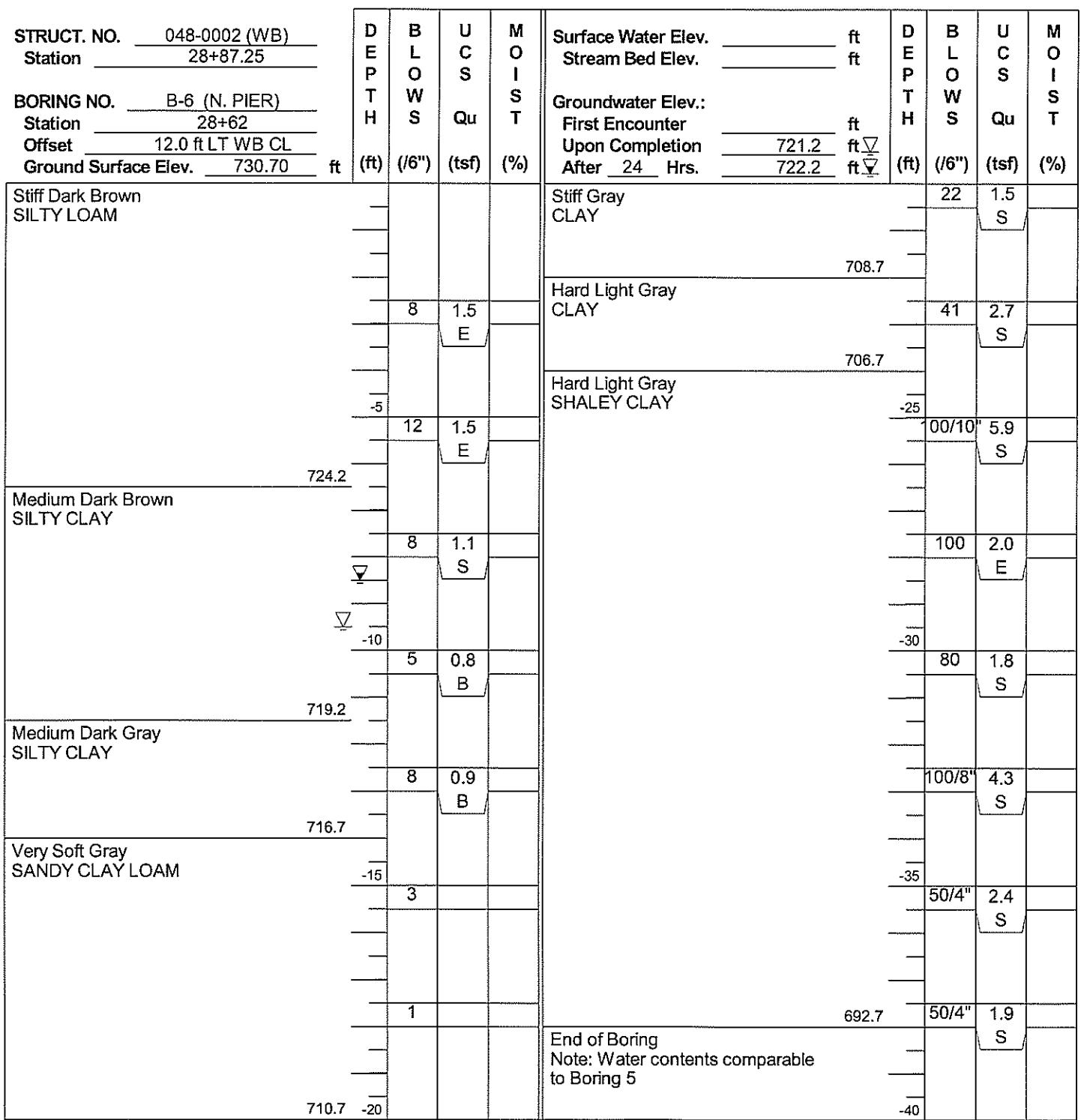
The Unconfined Compressive Strength (UCS) Failure Mode is indicated by (B-Bulge, S-Shear, P-Penetrometer). The SPT (N value) is the sum of the last two blow values in each sampling zone (AASHTO T206).
