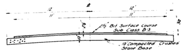
CROSS SECTION BITUMINOUS SURFACE
