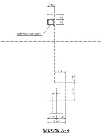
\* EPOXY GROUT BARS IN 9" MIN. HOLES ACCORDING TO ARTICLE 584 OF THE STANDARD SPECIFICATIONS.
