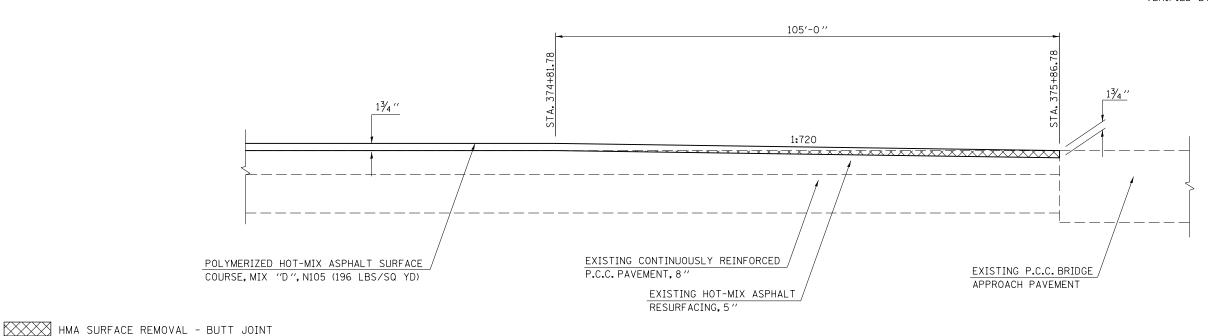
DETAIL FOR I-74 MILLING /PAVING TRANSITION AT S.N. 057-0134
