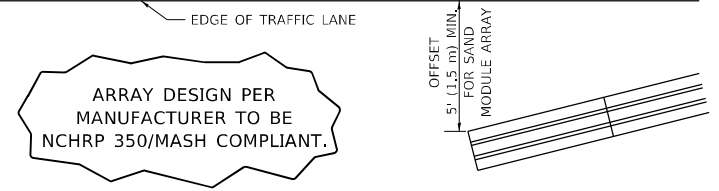
DETAIL "A" IMPACT ATTENUATOR, TEMPORARY (SEE NOTE 5)
