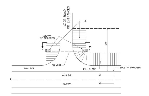
NOTE: ON A ONE-WAY FACILITY, THE GRATE ON THE DEPARTURE END IS NOT REQUIRED.
