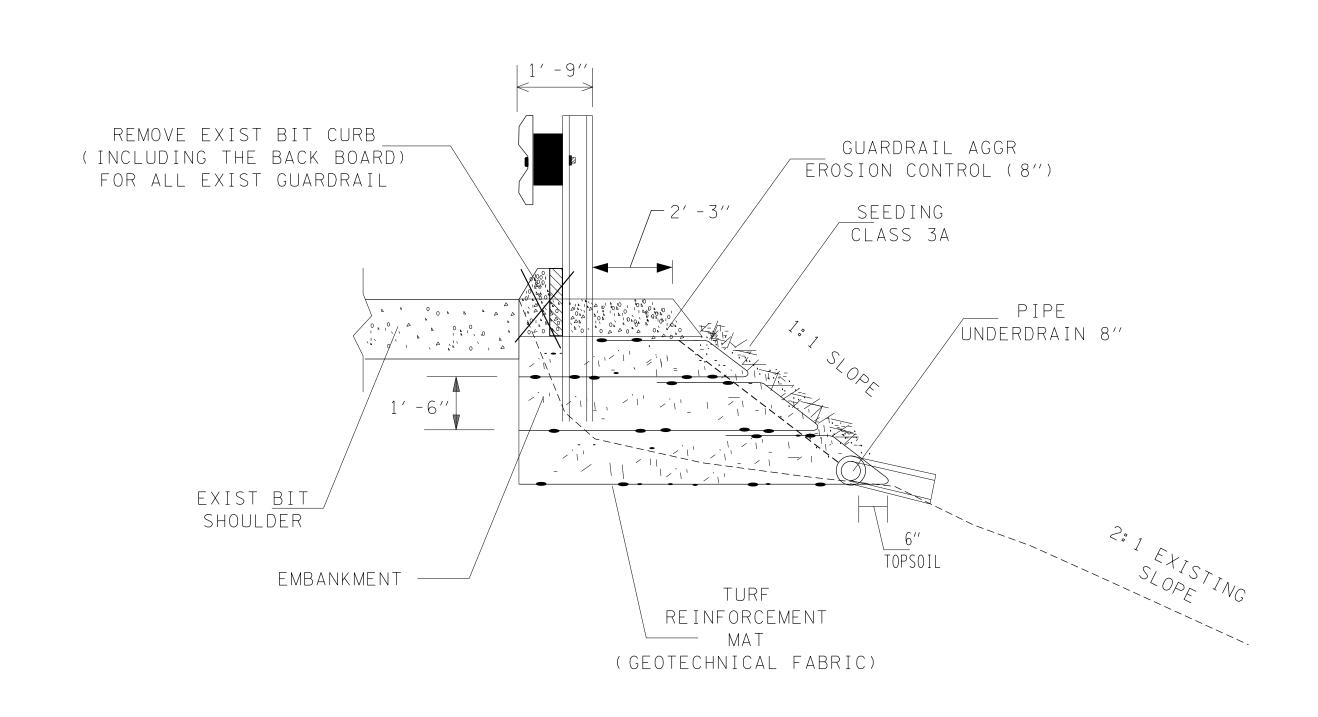
EARTH REIFORCEMENT DETAIL & TYPICAL SECTION
