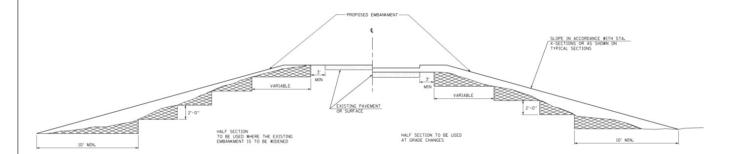
MATERIAL TO BE REMOVED AND REPLACED IN THE EMBANKMENT IN ACCORDANCE WITH ART. 205.04 OF THE STANDARD SPECIFICATION. COST TO BE INCLUDED IN THE VARIOUS ITEMS OF EXCAVATION AND NO ADDITIONAL COMPENSATION WILL BE ALLOWED BECAUSE OF THIS WORK.
