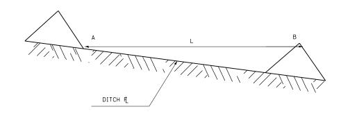
L = THE DISTANCE SUCH THAT POINTS A AND B ARE OF EQUAL ELEVATION
