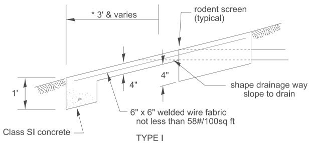
Outlets are to be constructed in accordance with applicable portions of Section 606 of the Standard Specifications.
