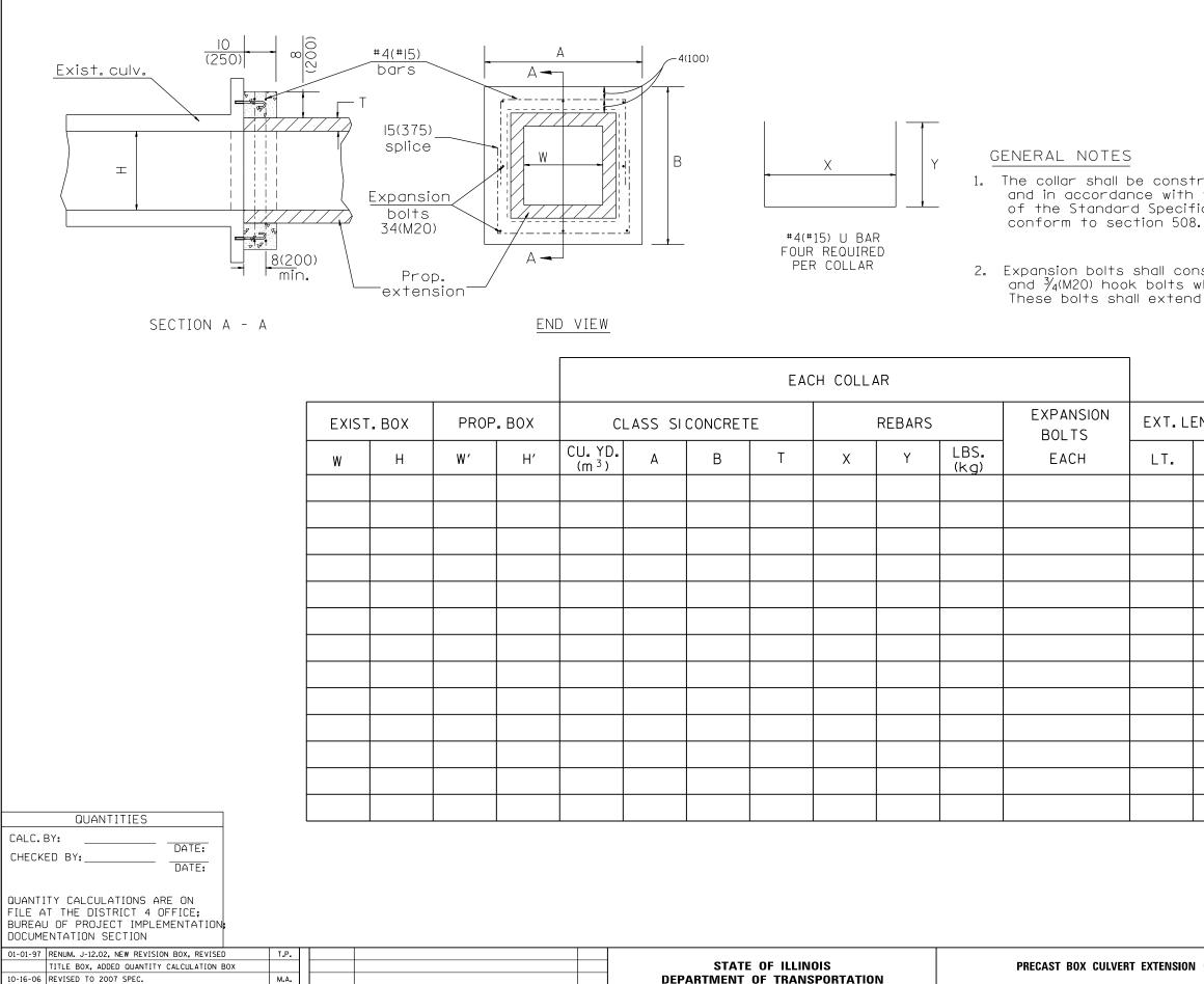
1. The collar shall be constructed entirely of CLASS SI CONCRETE and in accordance with the applicable portions of section 503 of the Standard Specifications. REINFORCEMENT BARS shall conform to section 508.
