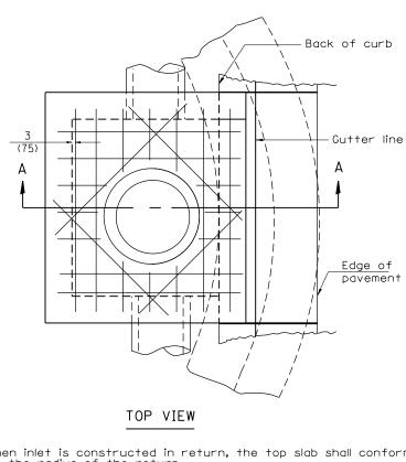
When inlet is constructed in return, the top slab shall conform to the radius of the return.
