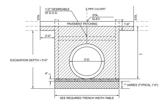
TRENCH PROTECTION REQUIRED WHEN EXCAVATION DEPTH EXCEEDS 5' SEE EXCAVATION DEPTHS TABLE FOR CONTRACTOR OPTIONAL CONFIGURATIONS
