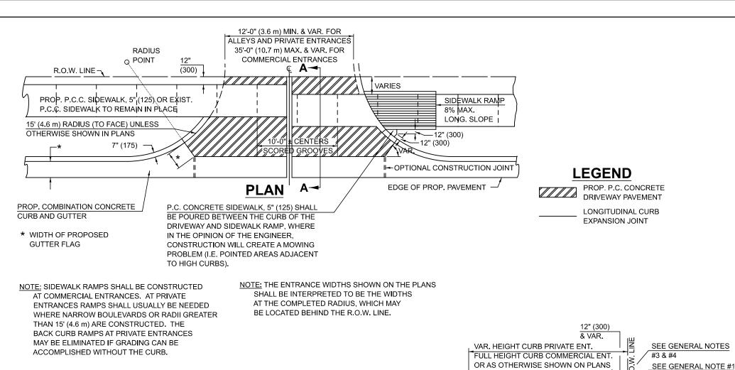
12" (300) CROSS SLOPE FOR SIDEWALK: & VAR. 1% (1/8" PER FT.) (MIN.) 2% (1/4" PER FT.) (MAX.) **SEE GENERAL NOTE #1** SEE NOTE #5 THICKNESS OF PROP. P.C. CONC. THICKNESS AS SIDEWALK SHALL BE THE SAME SPECIFIED 3'-0" THICKNESS AS THE P.C. CONC. IN THE PLANS (0.9 m)DRIVEWAY PAVEMENT PROPOSED COMBINATION CONCRETE CURB AND GUTTER (DEPRESSED)
