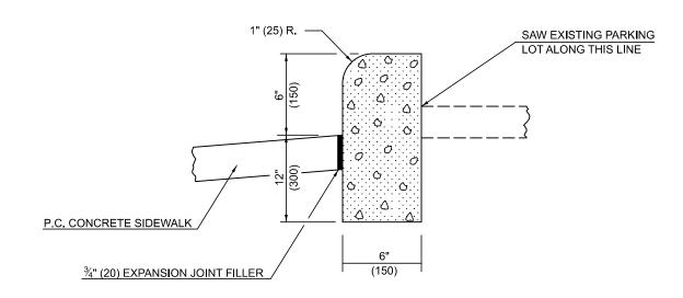
THE CONCRETE CURB, TYPE B, SHALL BE CONSTRUCTED FROM CLASS SI CONCRETE THROUGHOUT. THIS WORK WILL BE PAID FOR AT THE CONTRACT UNIT PRICE PER LINEAL FOOT (METER), FOR CONCRETE CURB, TYPE B, WHICH PRICE SHALL INCLUDE ALL MATERIALS AND LABOR NECESSARY TO COMPLETE THE WORK.
