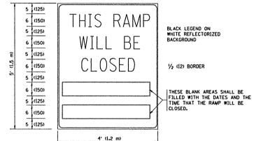
THESE SIGNS ARE REQUIRED ON BOTH SIDES OF THE RAMP, MINIMUM OF I WEEK IN ADVANCE OF THE CLOSURE.
