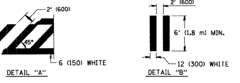
TYPICAL CROSSWALK MARKING
