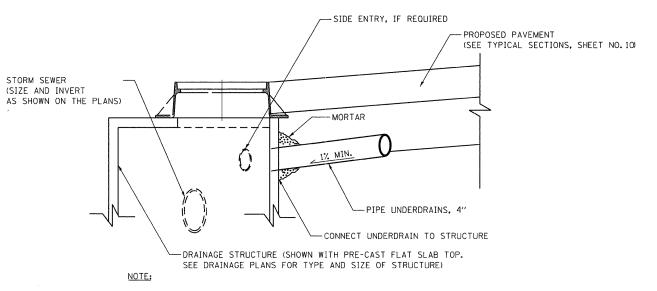
THE CONTRACTOR SHALL CAREFULLY CORE INTO THE DRAINAGE STRUCTURE THE SAME SIZE AS THE EXTERNAL DIAMETER OF THE PROPOSED PIPE UNDERDRAIN. THE PROTRUSION OF THE PROPOSED PIPE UNDERDRAIN INTO THE DRAINAGE STRUCTURE MUST NOT EXCEED A MAXIMUM OF ONE INCH. AFTER THE PIPE UNDERDRAIN IS INSTALLED, THE DRAINAGE STRUCTURE SHALL BE MORTARED WITH A NON-SHRINK CONCRETE GROUT.
