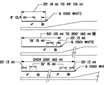
FULL SIZE LETTERS 8' (2.4 m) AND ARROWS SHALL BE USED.  $\P$  AREA = 15.6 SO. FT. (1.5 m<sup>2</sup> )  $ML^{\gamma}$  AREA = 20.8 SO. FT. (1.9 m<sup>2</sup>)
