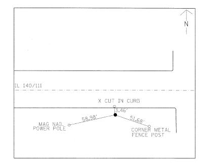
CONTROL PT 505 REBAR WITH IDOT CAP STA. 464+26.99 38.77 RT N 815,180.1354 E 321,383.0032
