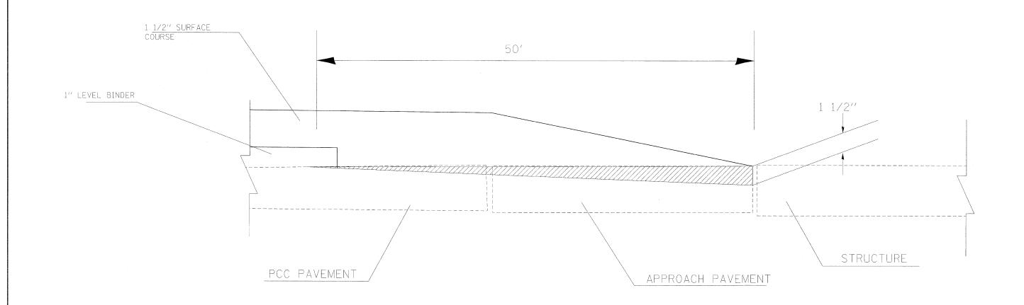
PCC & HMA SURFACE REMOVAL - BUTT JOINT
