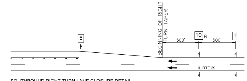
SOUTHBOUND RIGHT TURN LANE CLOSURE DETAIL
