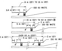
\* TURN LANES IN EXCESS OF 120 m (400') IN LENGTH MAY HAVE AN ADDITIONAL SET OF ARROW - "ONLY" INSTALLED MIDWAY BETWEEN THE OTHER TWO SETS OF
