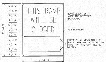
THESE SIGNS ARE REQUIRED ON BOTH SIDES OF THE RAMP, MINIMUM OF I WEEK IN ADVANCE OF THE CLOSURE.
